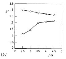
Figure 1: Capacity factor variation of nitrate and nitrite with: a) ionic strength and b) pH. Column: Partisil SAX (250x4.6 mm i.d., 10  $\mu$ m). Mobile phase: 0.03M  $KH_2PO_4/H_3PO_4$ , pH 3.5. Flow-rate: 1.5 mL.min<sup>-1</sup>.  $\lambda_{det}$  = 210 nm.
